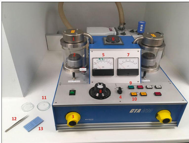
Fig. 2 CTA 010 glow discharger and required materials. Relevant elements are numbered: (1) Chamber metal lid, (2) glass vacuum chamber, (3) vacuum knob, (4) chamber knob, (5) pressure gauge, (6) timer, (7) current gauge, (8) voltage dial, (9) start button, (10) vent button, (11) petri dish with filter paper and grid, (12) metal tweezers, (13) grid box
